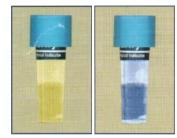
h. If you see this result, then the autoclave is operating correctly. If this is not the result attained, please contact the IM Laboratory Supervisor immediately. Discard both ampules in the provided sharps container after results have been collected.
